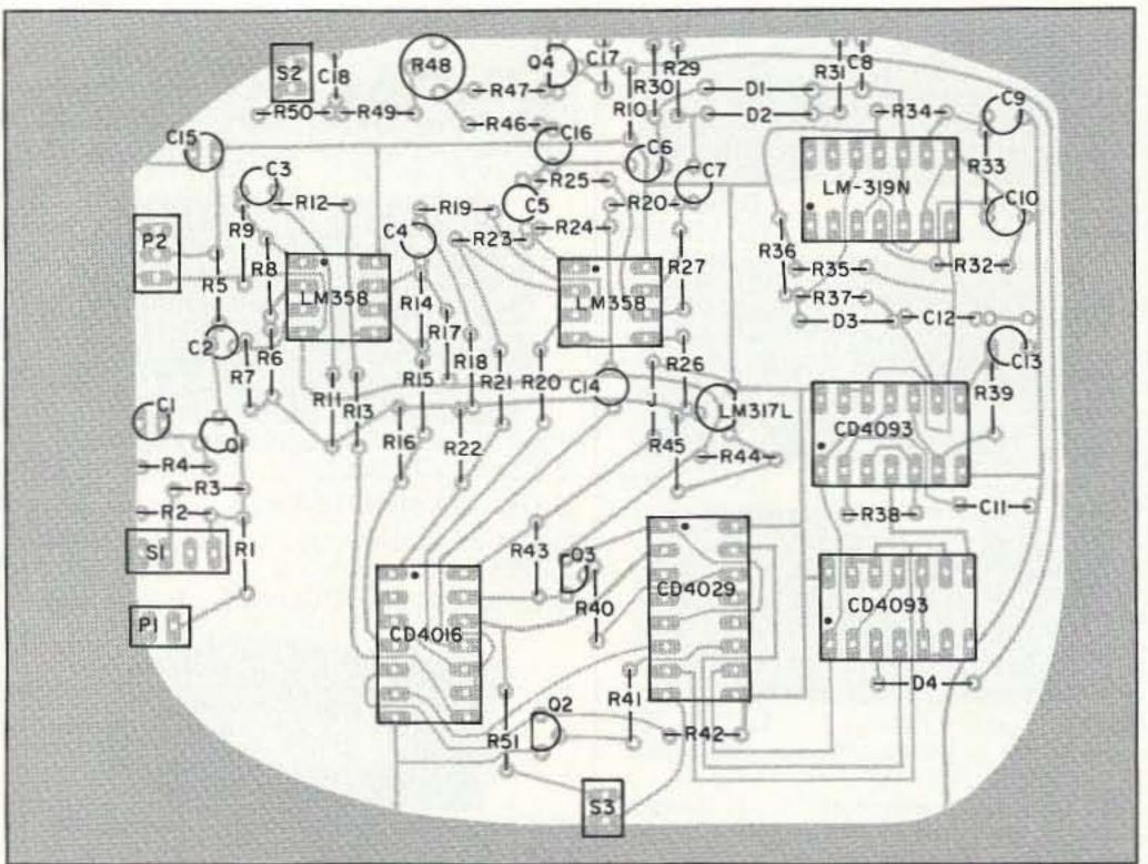
Figure 5b. PC board parts layout.
